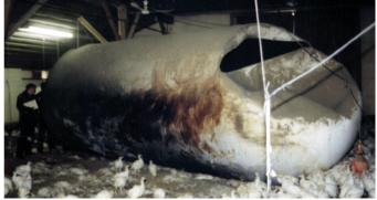
Left, Herrig Bros. 42-foot long tank before explosion. The tank was out in the open away from any buildings, and the tank and above ground piping had no protective fence to keep intruders away. Right, large tank fragment, about half of the tank, was propelled inside a turkey barn as a result of the explosion.
